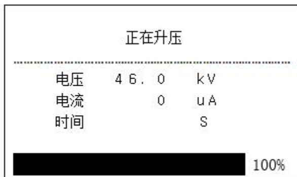
FIG. 20 Booster interface of automatic withstand voltage test
